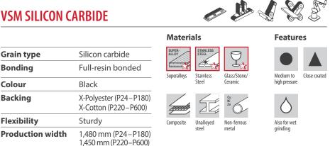
Universal silicon carbide abrasive on sturdy polyester/cotton cloth backing. CK721X is characterised by its superior grinding ability and a fine surface finish. It is also oil- and waterproof, and is especially suitable for working on mineral materials.
